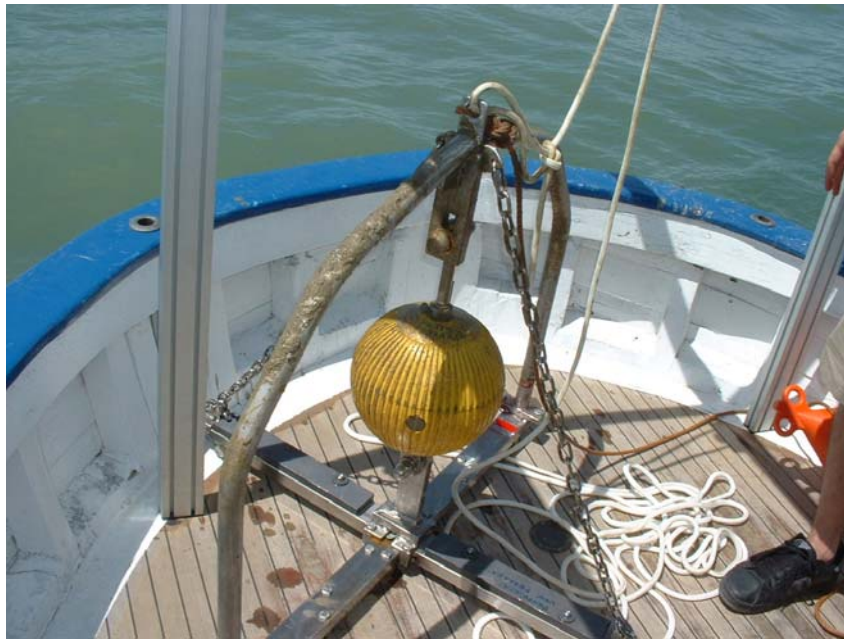
Fig. 4. View of one of the directional wave gauges after retrieval for maintenance
